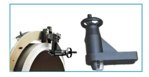
Performs counter boring Tool Feed: Manually Max. Travel: 70mm
